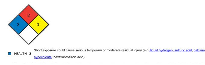
Must be moderately heated or exposed to relatively high ambient temperature before ignition can occur and multiple finely
