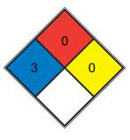
Short exposure could cause serious temporary or moderate residual injury (e.g. <u>liquid hydrogen, sulfuric acid, calcium</u>
